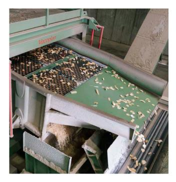
In addition to high-performance shredders, grinders, and chippers, Vecoplan manufactures a wide range of equipment for a complete plant solution. Screening, separation, storage, dosing equipment, and more can be tailored to meet virtually any processing need.
